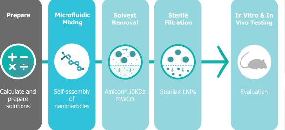
**Manufacturing Parameters - Ignite settings:** Total Flow Rate: 20 mL/min Flow Rate Ratio (Aqueous:Organic): 3:1
