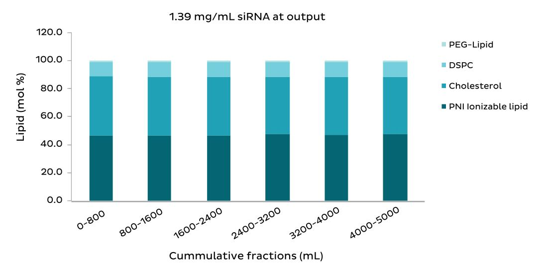
Composition of siRNA LNPs were consitent between fractions collected from 5L continuous flow manufacturing run on the 8x Scale-Up system. LNPs were disrupted and lipids were separated and analyzed on an HPLC column using ELS detector.
