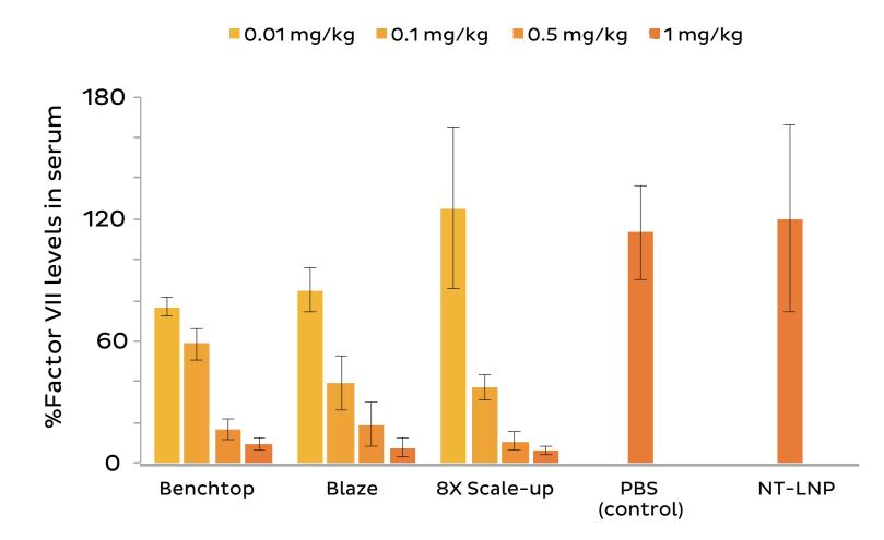
LNPs containing siRNA against FVII or non-targeting (NT) control were administered to CD1 mice by tail vein injection at the doses indicated. Knockdown efficacy was maintained between LNPs produced on the NanoAssemblr Benchtop, Blaze and 8x Scale-up at 10, 100, and 1000 mL batches respectively.
