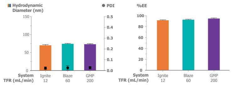
Particle size, polydispersity and RNA encapsulation efficiency are consistent as production of epo-encoded mRNA-lipid nanoparticles (LNPs) was scaled using the NanoAssemblr platform.
